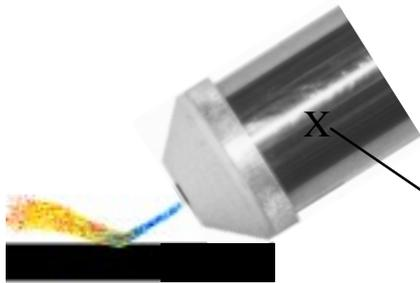
Initiate the pilot arc and lay the torch over at approximately 60°
