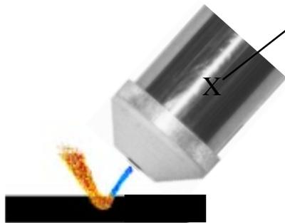
Begin twisting the torch slowly towards a vertical position taking care to avoid ejected material from hitting the nozzle. At the same time, the torch should be moved a small distance along the work piece.
