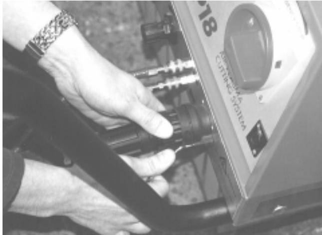
Note that a sealing ring is located in the base of the torch connector socket to form an air seal with the centre power pin. Care should be taken to ensure that this seal is not displaced and that the end of the pin is not damaged when the torch plug is removed.
