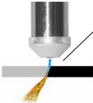
Under normal cutting conditions the torch is designed to operate with a STAND OFF of about 6 mm. This is the distance between the end of the nozzle and the work piece.
